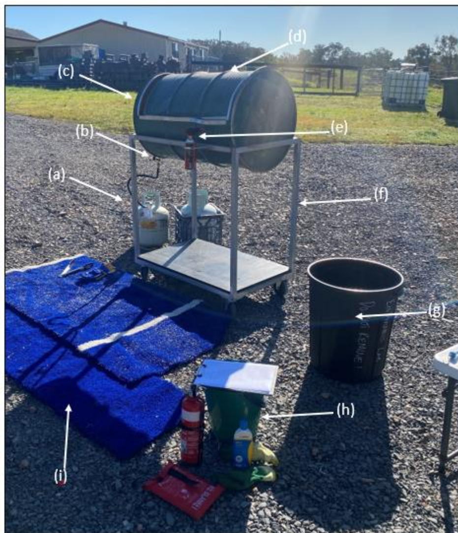
Fig. 2.3 The shoot flammability device used in this research: (a) gas cylinder, (b) gas flow tap, (c) device tub housing grill, (d) moveable wind protection hood, (e) butane blowtorch, (f) portable stand on lockable wheels, (g) tub filled with water to
