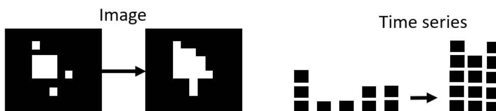
FIGURE 5 The application of dilation operation to an image and time series
