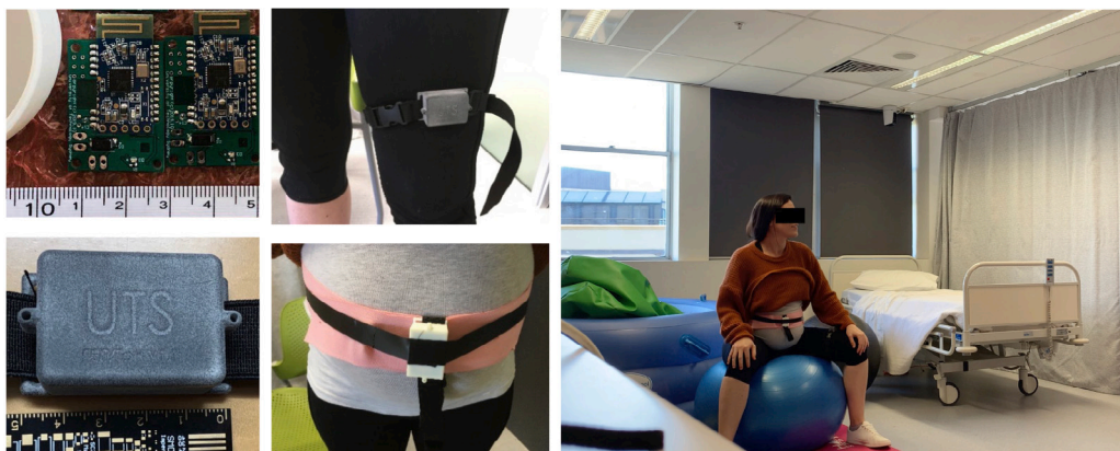
(a) Designed wearable (b) The mobilisation monitoring of woman experiencing high risk pregnancy in a motion tracking device. pilot study. The devices are attached on the left thigh and in front of the abdomen.
