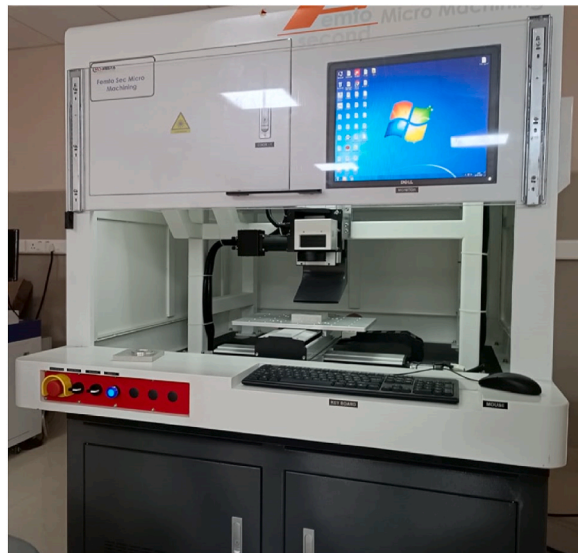
Fig. 3. Femtosecond laser micromachining center
