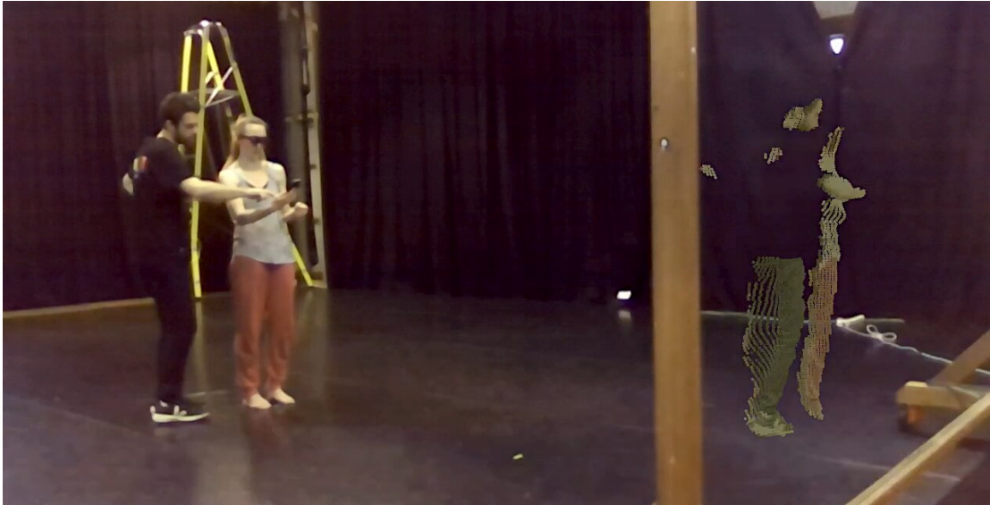
Figure 6.4. – My shirt as visible on the left does not appear in the capture from the Azure Kinect that appears in the mirror on the right.
