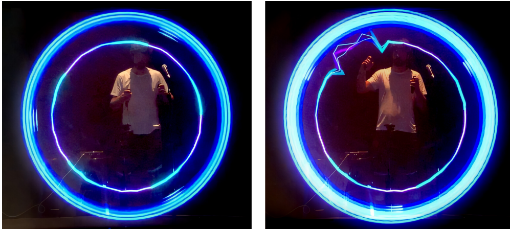
Figure 4.14. – The innermost circle in these images is The Ring, a membranous circle that vibrates when struck to produce electronic drum sounds.
