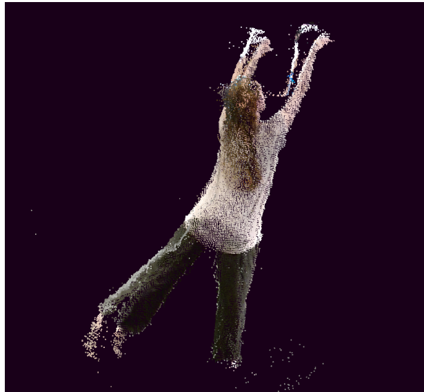
Figure 6.2. – The effect of unsynchronised shutters in a multi-camera array. Notice the artefacts around the arms and legs as the dancer moves at speed.
