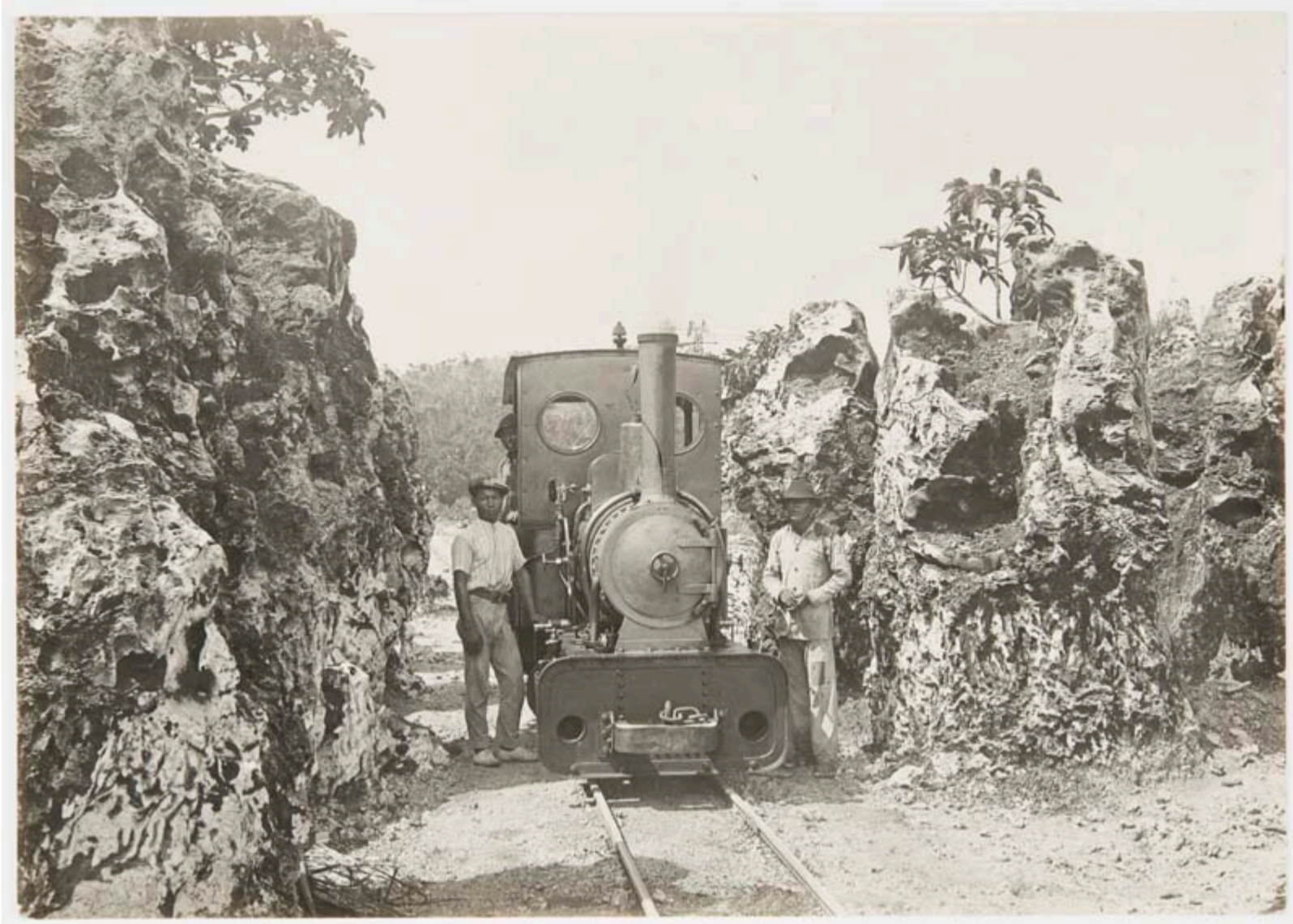
Fig. 23. The locomotives used to shunt phosphate carts from the mining sites to the loading facilities on Nauru were imported from Britain and Germany. Shown here is a steam locomotive in c.1915. The island's aerial cableway can be seen in the background of the image. Maslyn Williams Nauru Photographs, State Library of New South Wales, PXB 293, Image 69.
