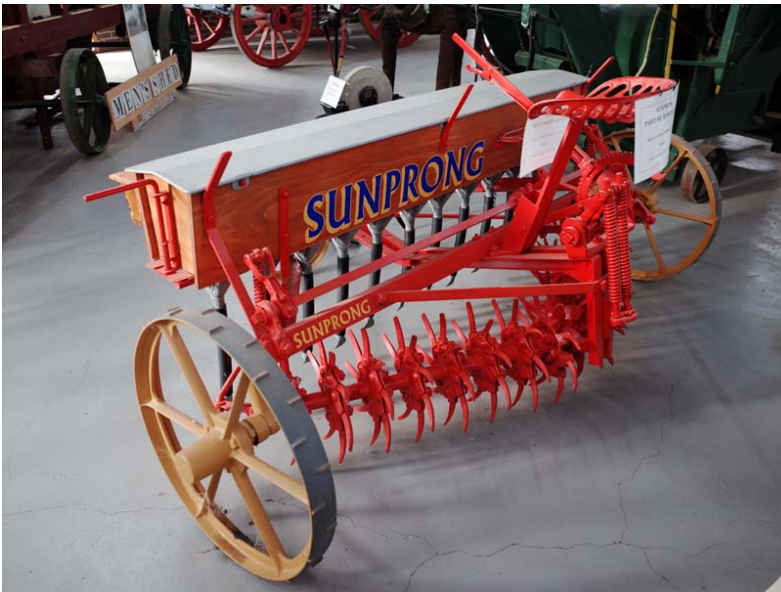
Fig. 35. The Sunprong Pasture Renovator, manufactured at the Sunshine Harvester Works in c.1935. Doses of superphosphate are dropped onto the ground before the rotating prongs turn over the topsoil, mixing in the fertilizer.
