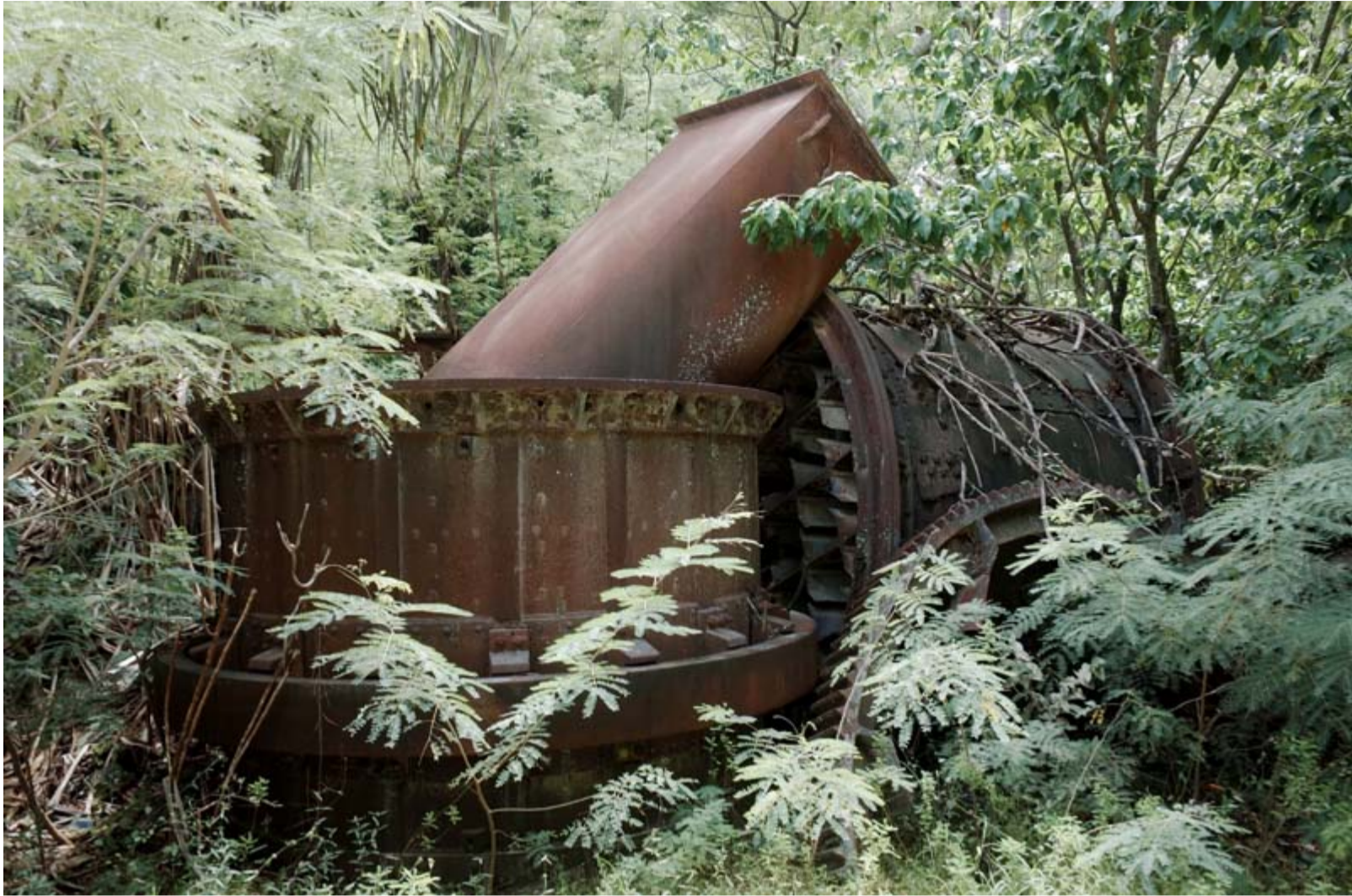
Fig. 25. Parts of the twentieth-century industrial equipment used to process phosphate remain dispersed around Nauru today. Seen here are likely the elements of a rotatory drying system, used to prepare the crushed phosphate prior to shipping according to international industry standards regarding moisture content.
