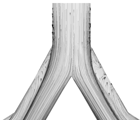
Figure 9. Separation of streamlines and generation of secondary vortices on the symmetric plane at the bifurcation region of G3.
