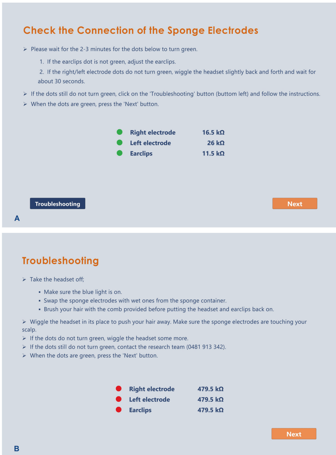
Fig. 2 Impedance verification instructions. A Participants will be instructed to check the electrodes impedance connection. If participants encounter issues to turn the impedance indicators green ( < 50 \text{ k}\Omega ), they will be guided to press the troubleshooting button, prompting access to the troubleshooting screen. B In the troubleshooting screen, they will be led through some simple steps to resolve the issue.
