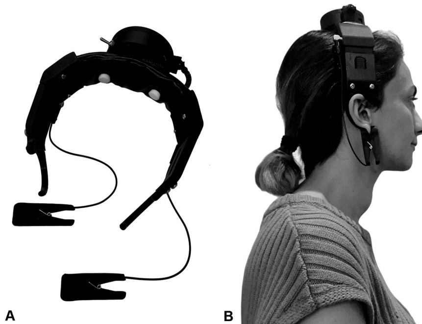
Fig. 1 The in-house-developed EEG headset. A The headset is equipped with an OpenBCI biosensing board, with two sensors at C3 and C4 electrode sites, and ear-clips serving as the reference electrodes. B The placement of the EEG headset on the head.
