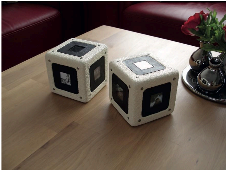
Figure 1: The Cueb system consists of two cubes that each contain six displays for showing a person's digital photos (Golsteijn & van den Hoven, 2013). Photo: Connie Golsteijn. [ALT TEXT: The photo shows the Cueb system, with two Cueb devices sitting on a tabletop. Each Cueb device has six displays, one on each side, that are used to show a person's digital photos.]
