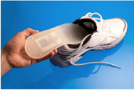
Fig. 21. Photograph of the printed wireless pressure and temperature sensor within a shoe's insole [156].
