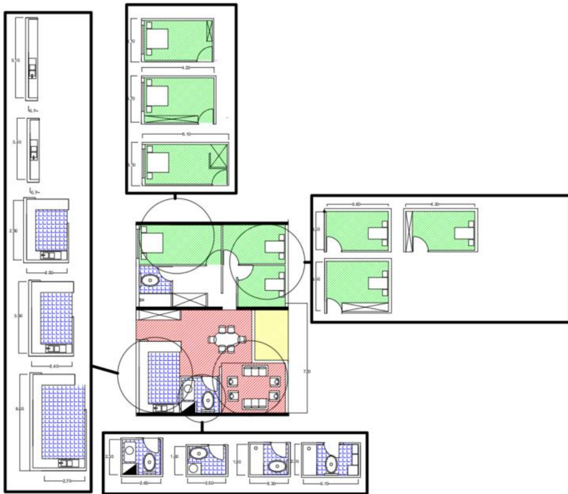
Figure 46- A schematic view of an apartment plan and the dominant dimensions of spatial voids based on the cluster analysis results
