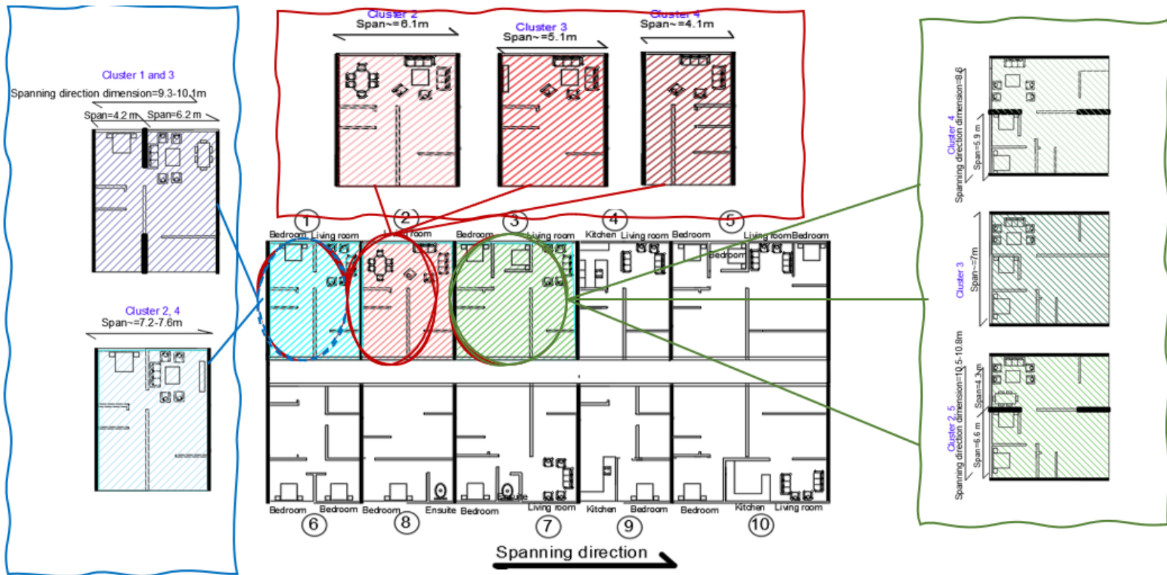
Figure 55- A schematic view modular design scenario based on recognising the manufacturability of layout design and finding a pattern according to the similarities of architectural design
