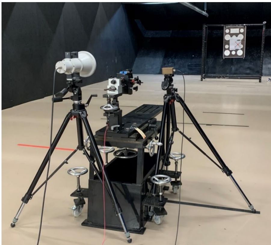
Figure 3-14: Chronograph and firearm set up aimed perpendicularly at the target (10 m distance between muzzle and target), in an indoor firing range.
