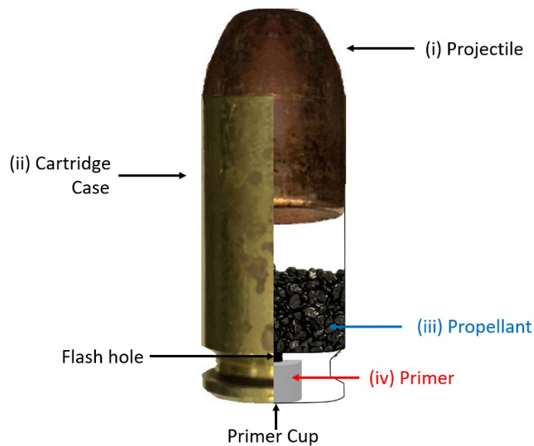
Figure 1-1: Diagram of FEDERAL® .40 S&W ammunition.
