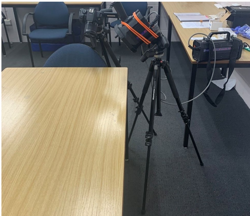
Figure 3-2: UV light source and camera set up to visualise and photograph shooter's hand and firearm post discharge.
