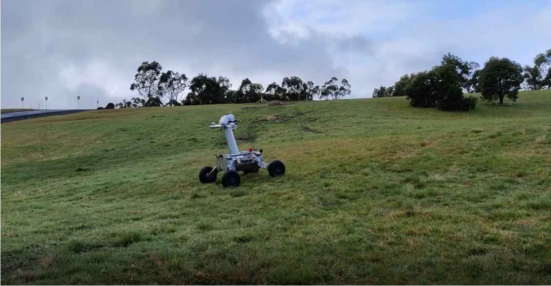
FIGURE 1.1: Outdoor Robotic Platform designed for operation in challenging outdoor environments. The FORV (Fast Off-road Vehicle) developed at UTS, is the experimental platform used in this work.
