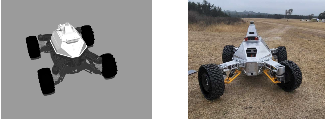
FIGURE 5.1: The FORV 2 developed at UTS in (a) simulation and (b) hardware.
