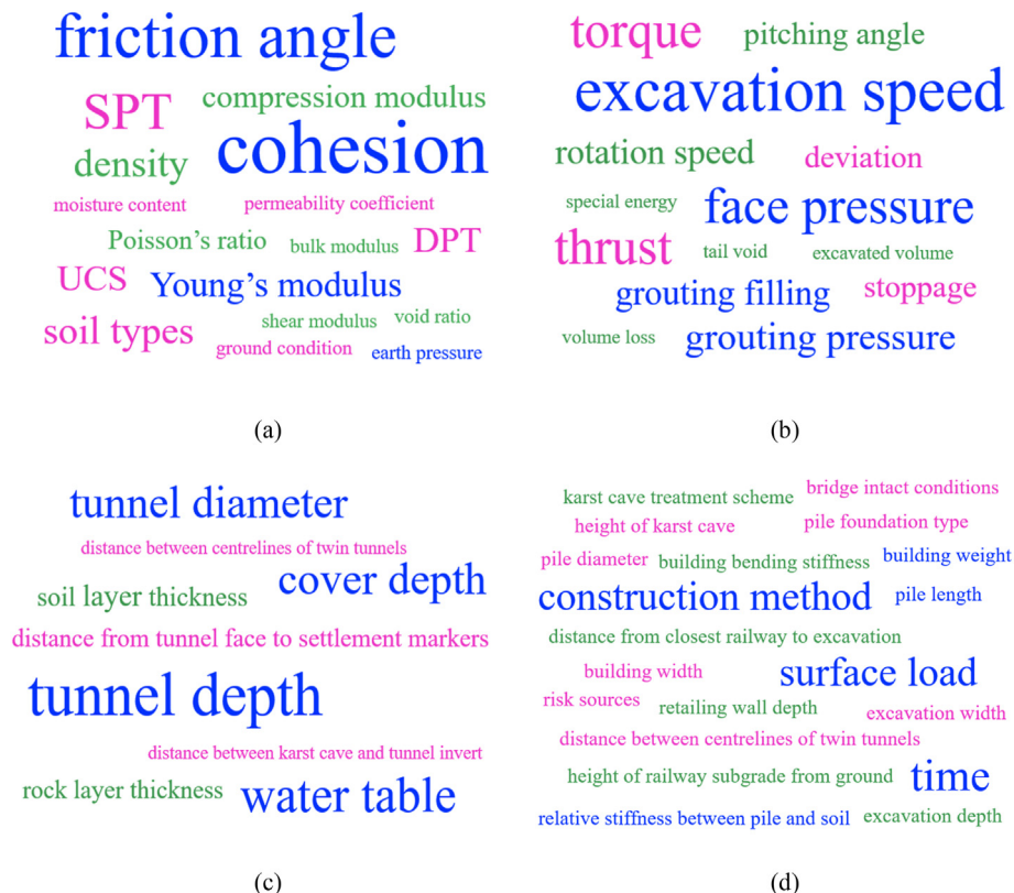
Fig. 13. Influencing factors of GSS caused by tunnelling. (a) geotechnical parameters (b) TBM operation parameters (c) tunnel geometry and (d) other factors.
