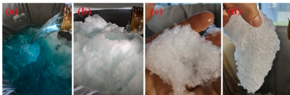
Fig. 10. FC of electroplating wastewater for water purification and heavy metal removal. Taken from [291].
