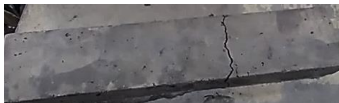
Figure 9. The image of the sample after the flexural strength test.
