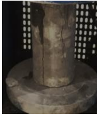
Figure 6. The image of the sample after the compressive strength test.
