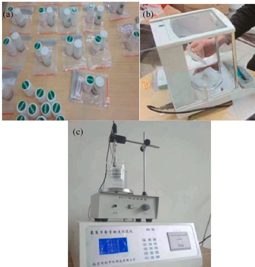
Fig. 5. Chlorine ion concentration measurement process(a) the concrete powder (b) weighing the powder(c) test the chloride ions.
