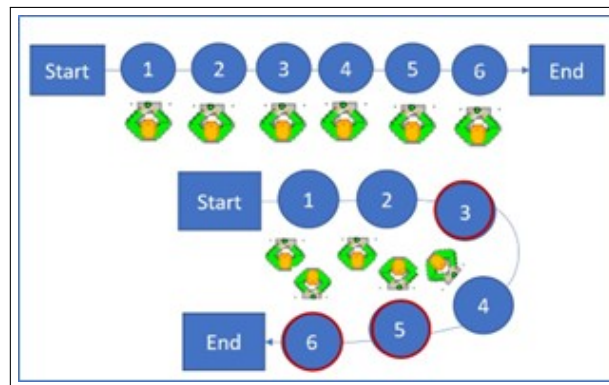
Figure 5.10: Straight and U-shaped assembly line
