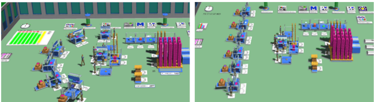
Figure 6. Tecnomatix 3D model for both layouts: curved (left), linear (right)
