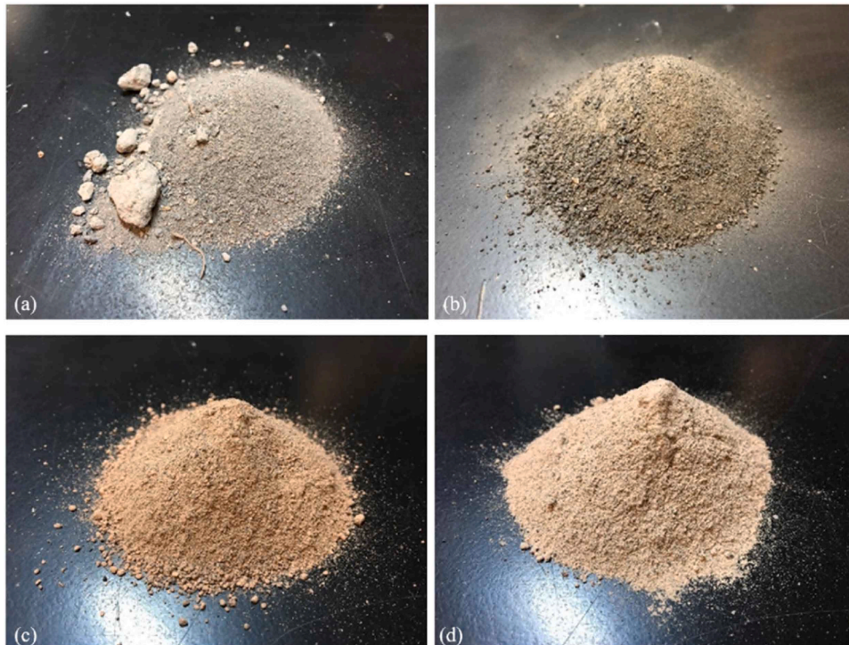
Fig. 9. Lunar regolith and Martian soil simulants: (a) BP-1 lunar simulant [56], (b) JSC-1A lunar simulant [57], (c) MGS-1 Mars global simulant [58], and (d) MGS-1C Mars global simulant enriched with smectite [58].
