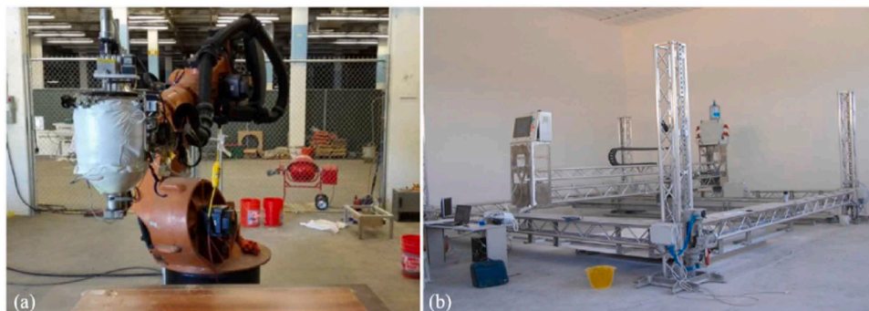
Fig. 33. (a) Contour Crafting 3D printer [124] and (b) D-shape 3D printer [204].
