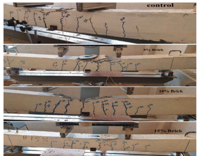
Fig. 26. Failure mode of beams containing broken bricks [143].
