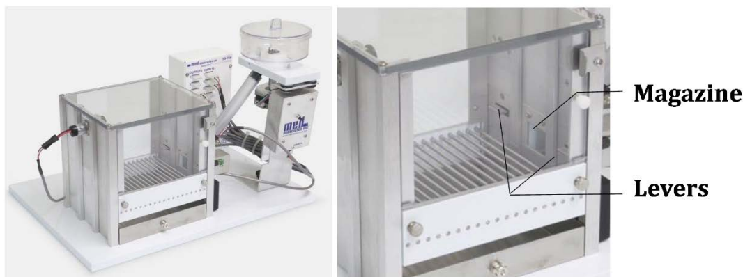
Figure 4.2: Pictorial representation of outcome devaluation chamber.
