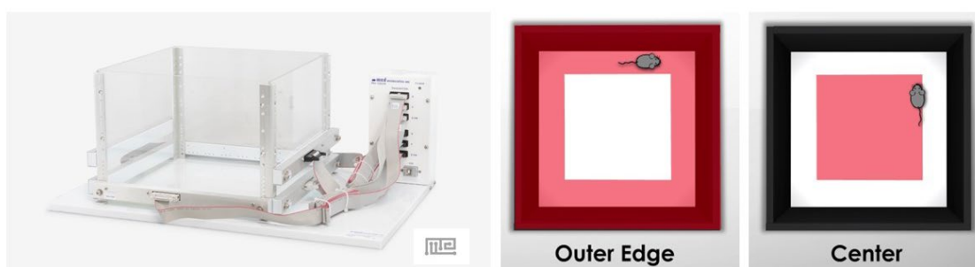
Figure 3.1: OFT chamber used for this experiment (left), an example of how the open field is split into outer edge and centre zone for analysis (right).
