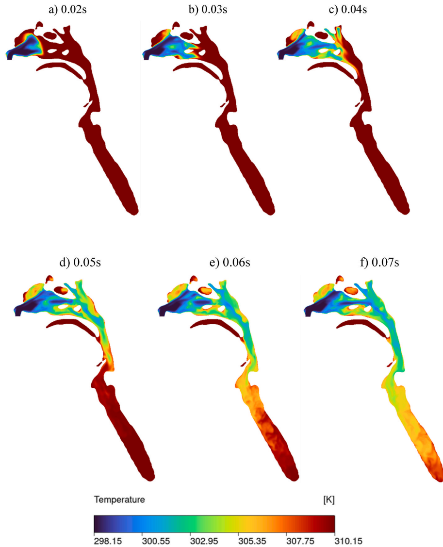
Fig. 6. Temperature (K) contour within the central cross-sectional plane of the upper airway from 0.02 to 0.07 s in the 298.15 K air inhalation simulation, illustrating dynamic thermal changes.
