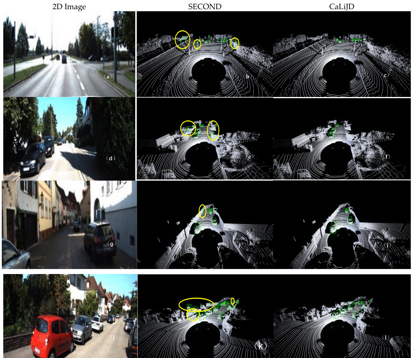
Figure 7. Visualization of the KITTI dataset. (a,d,g,j) show 2D images from four different scenes. (b,e,h,k) present the visualizations of 3D detection using the SECOND for these four scenes. (c,f,i,l) show the visualization results for the CaLiJD. The green 3D bounding boxes represent the detection results, whereas the areas within the yellow circles indicate the erroneous detections.
