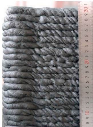
Fig. 6. Buildability test by layer deformation method [67].
