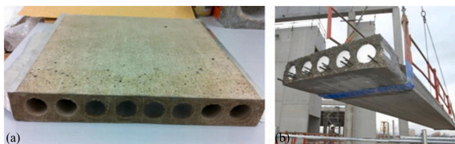
Fig. 17. (a) Standard concrete floor panels and (b) PCM-enhanced concrete floor panels [132].
