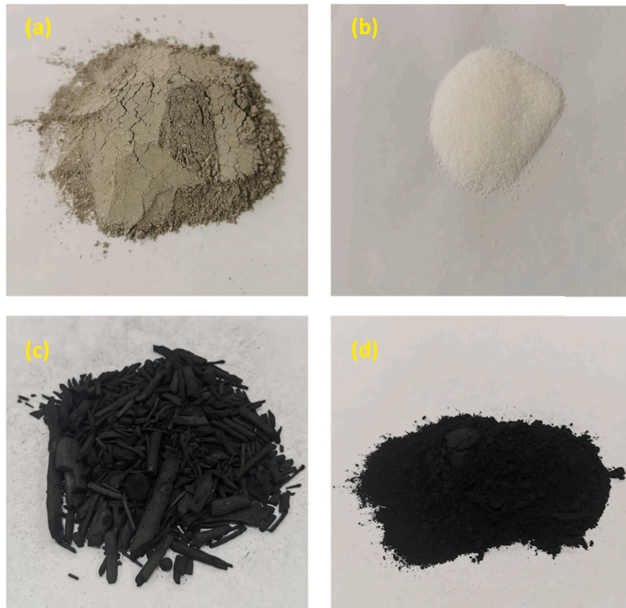
Fig. 1. Morphology of raw materials: (a) PENETRON CA, (b) SAP, (c) Original blended biochar, and (d) WWB.
