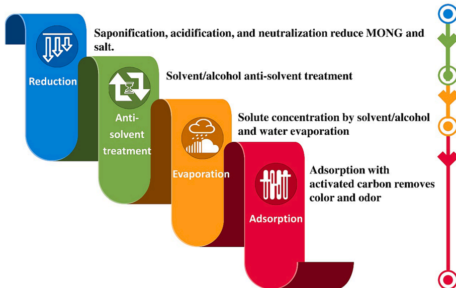
Fig. 9. Conventional refining steps for purification.
