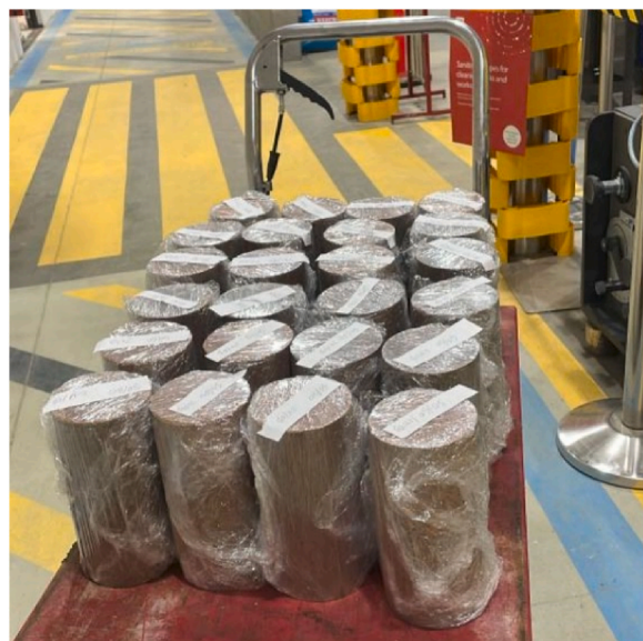
Fig. 4. Alkali-activated concrete samples sealed.
