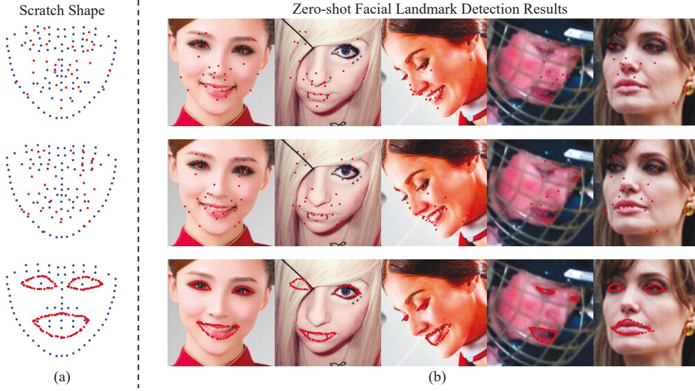
Figure 6.4: (a) the red points indicate the randomly generated scratch shape, and the blue points represent the mean shape of 98 landmarks, which serves as anchors during training. (b) the red points represent the zero-shot facial landmark detection results under various conditions.
