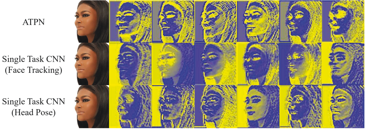
Figure 3.4: Column 1 shows the input image and column 2-7 are the low-level feature maps in the ATPN and two single task CNNs for head pose estimation and face tracking respectively. ATPN and the two single task CNNs utilize the same backbone for feature extraction. All visualized feature maps are from the 4-th MobileNet V3 block, and their resolution is 28 \times 28 . The pixel intensity of these feature maps represents the response strength of the corresponding pixel to the target tasks.
