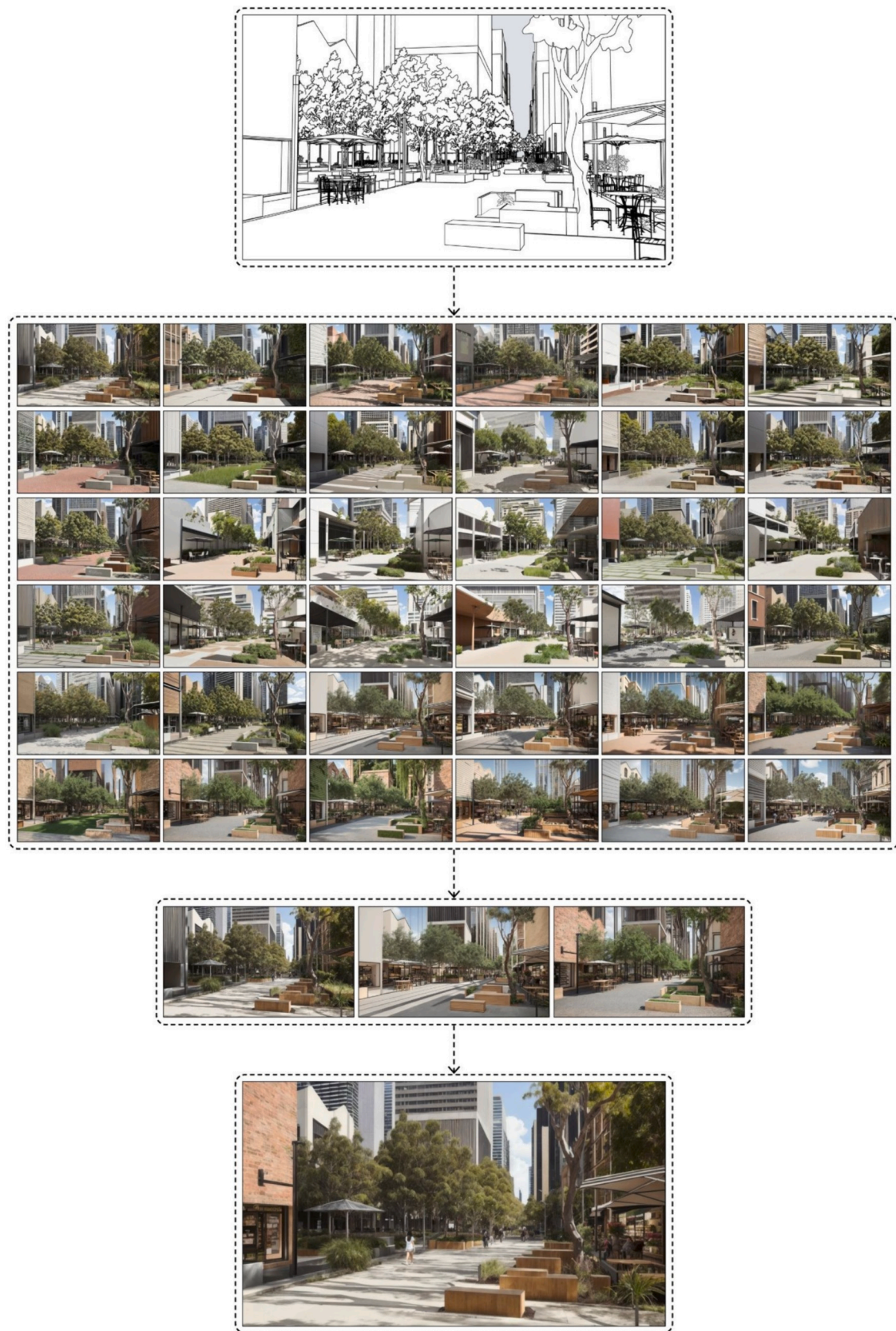
Fig. 25. The process of using ai (stable diffusion) to convert a sketch extracted from the 3d model to the final render used for visualisation.
