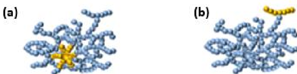
Figure 2. 14 schematic figure illustrate (a) high connected ligament to the network and (b) single connected ligament to the structure of the nanoporous network (Ron et al., 2020).
