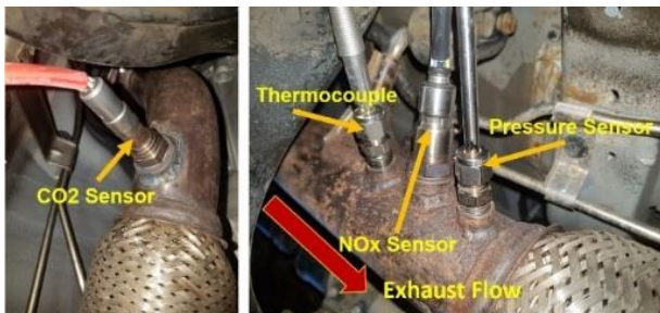
Figure 2. The installed sensors in the tested vehicle exhaust line.
