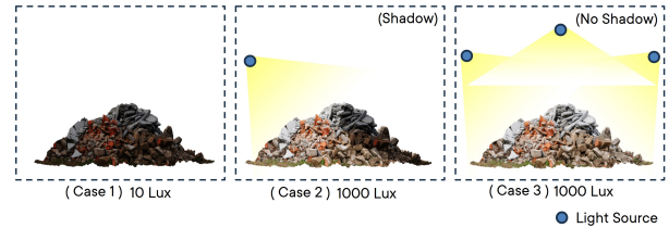
Figure 8. (Case 1) Experimental setup for 0 lux lighting, (Case 2) 1000 lux with a single-point light source, and (Case 3) 1000 lux with a three-point light source.
