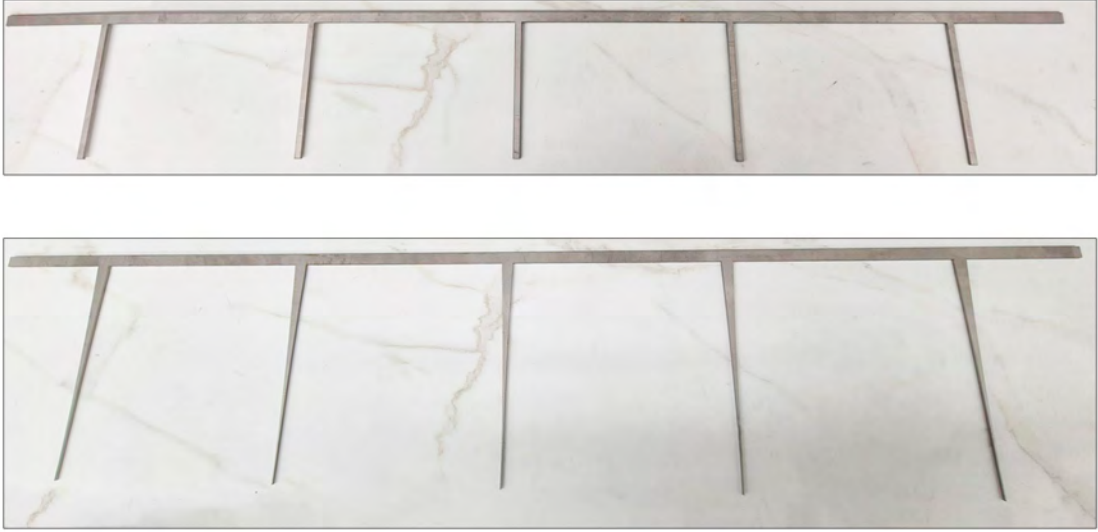
FIGURE 5.4: Fabricated stiffened beams. Top figure presents the rectangular-stiffened beam, and bottom figure presents the ABH-stiffened beam.
