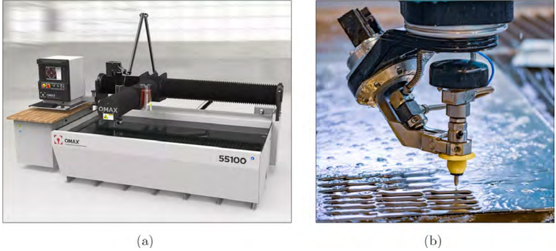
FIGURE 5.3: (a) The OMAX 55100 JetMachining Center utilized to fabricate the beams with rectangular and ABH stiffeners at UTS Tech Lab, from Ref. [85] . (b) Waterjet machine in operation, from Ref. [1].
