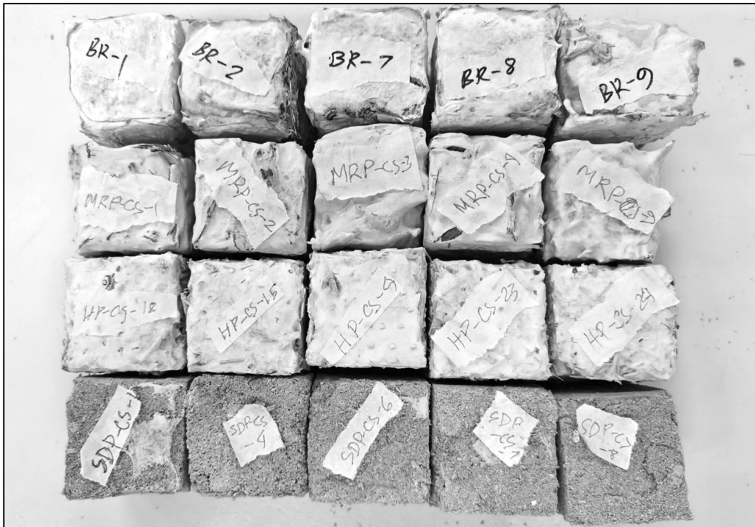
Figure 1(A) Methodology of bio-fabricating MBC samples; (B) MBC samples bio-fabricated with different substrates, where the first row is bagasse-based, the second row is Mulch-based, the third row is hemp-based, and the final row is sawdust-based MBC samples.
