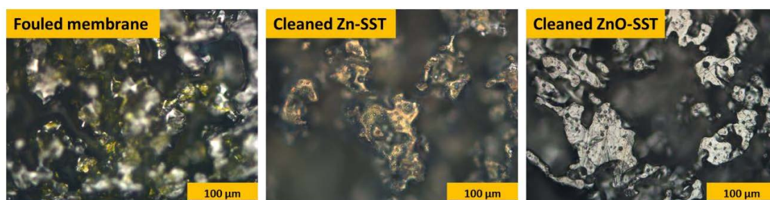
Figure 3.12. Optical microscope images of a fouled ZnO-SST membrane, and cleaned Zn-SST and ZnO-SST membranes after 30 minutes of UV light irradiation and water rinsing.
