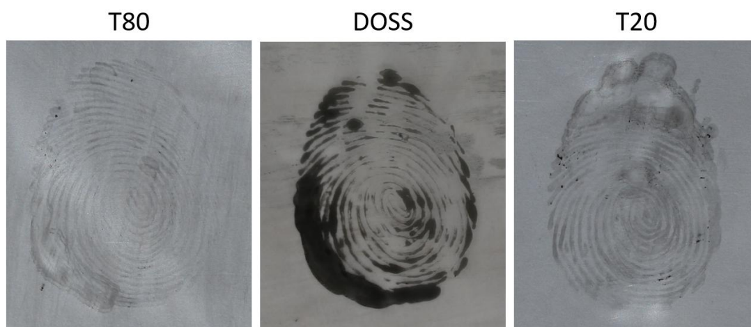
Figure 4.20 Examples of 'bubbling' produced by stamped sebaceous artificial residues on plastic substrate, developed using FePS made with T80, DOSS and T20
