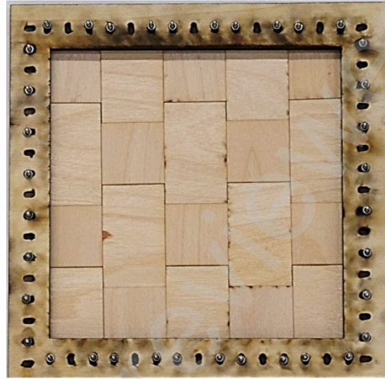
Figure 1: (A) Single-layer system of larch veneer strips, fixed at both ends, deflecting at RH = 90%. Bio-HNV small-scale prototype (B) front, (C) back of the panel. Overall panel size 180 mm x 180 mm, window size = 150 mm x 150 mm, Strip width 30 mm, Strip length = 160 mm, Strip thickness 0.6 mm.
