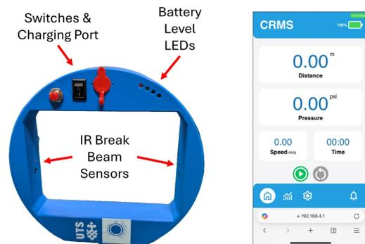
Figure 5: The remote monitoring system displays readings in real-time on the web-app user interface.
