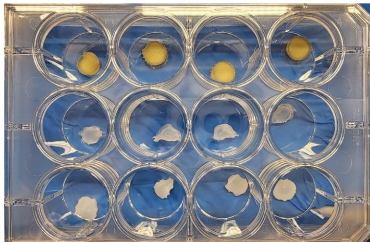
Figure 6-1 Photograph of the swelling test setup, showing 3 groups of hydrogel samples (superficial, middle, and deep layers), each with 4 replicates ( n = 4 ).
