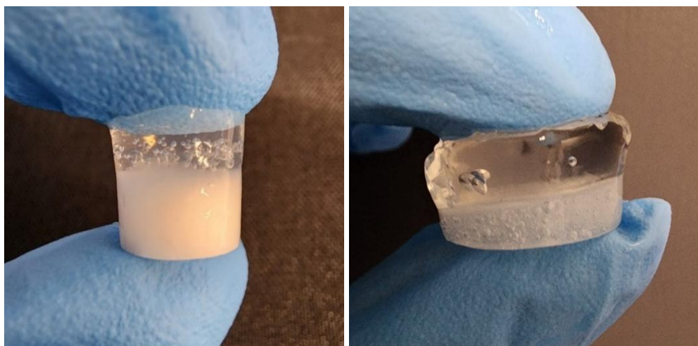
Figure 5-7 Alginate-based bilayered scaffold. The pure alginate hydrogel forms the cartilage layer, while the bottom mineralised layer was prepared using hydrogel material mixed with hydroxyapatite (HAp) (left) or bioactive glass (right).
