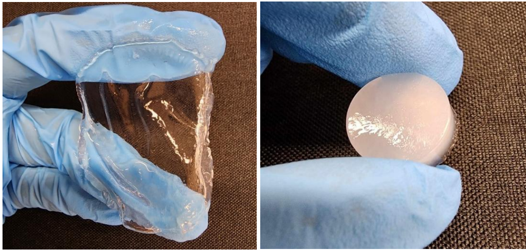
Figure 5-5 Pure PVA hydrogel in a thin layer (left) and a mould-casting thick hydrogel (right).
