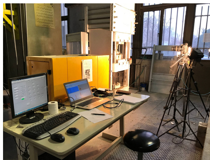
Figure 2. Test setup, including an acoustic emission system, for a compressive strength test.
