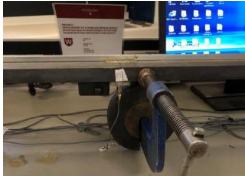
Figure 3-26 Adding 5 mass to the main beam
