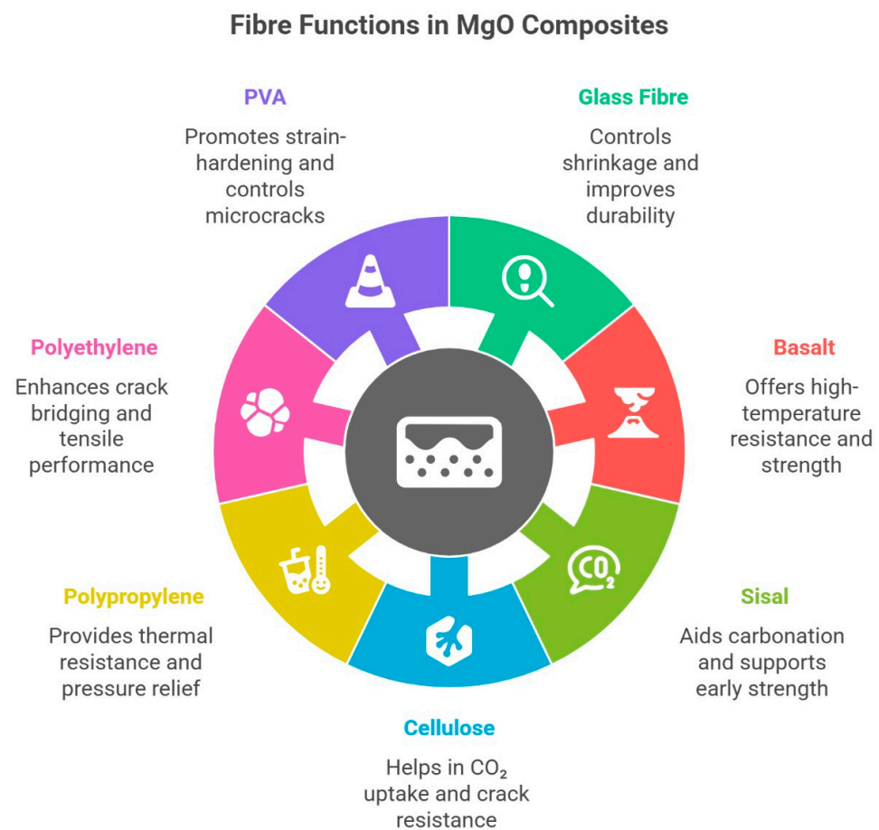
Figure 10. Fibre Functions in MgO Composites.
