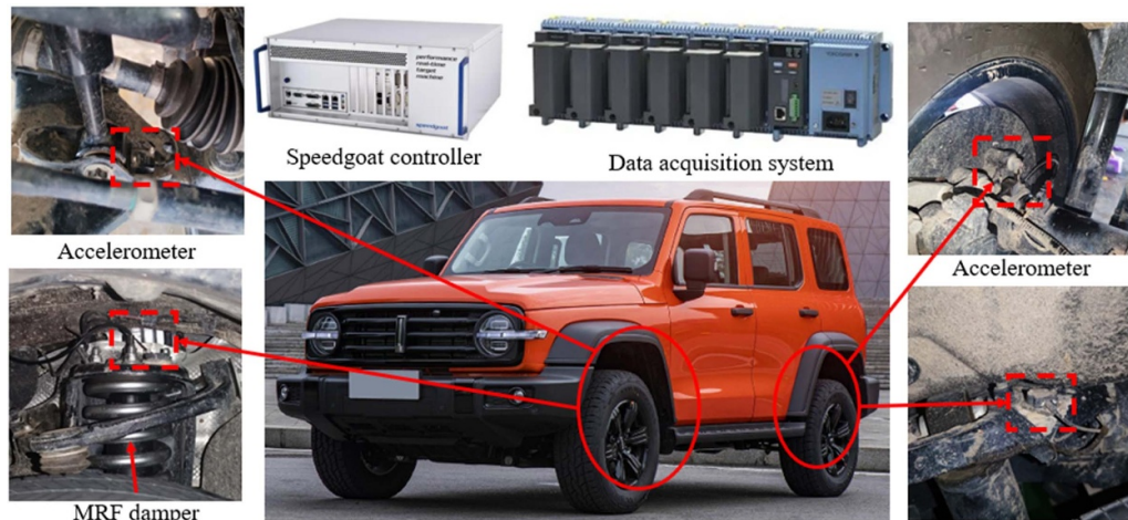
Figure 17. Instrumentation of full-vehicle MR suspension system.
