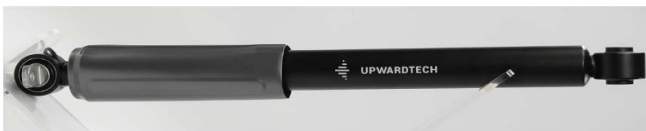
Figure 2. The manufactured MRF damper.
