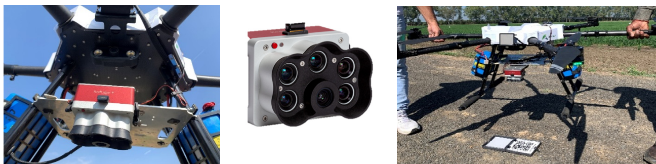
Figure 10. UAV-mounted with multispectral camera, sensor components, and calibration process. (In pic.: Multispectral camera model is MicaSense-RedEdge P and drone is Agribot by IOTech).
