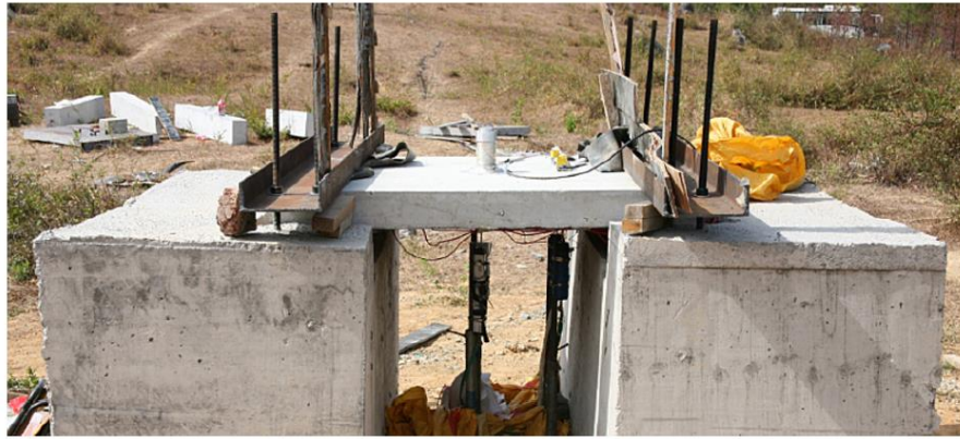
Figure 2.26. Illustration of contact charge test setup (Zhu et al., 2024)
