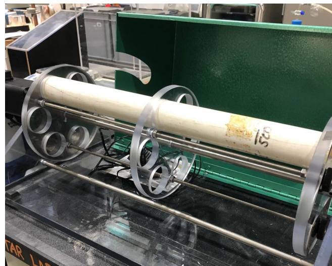
Figure 1. Rotation device for the autogenous shrinkage samples for the first 24 h.
