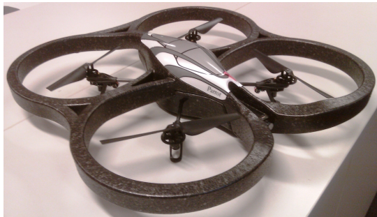
Figure 2: AR Drone Quadrotor used to collect the first data set
