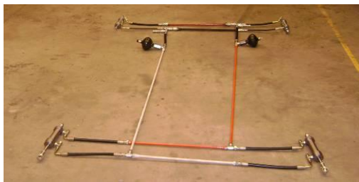
Figure 5 the assembled HIS system
