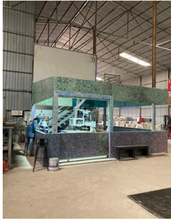
Photo 9. Converting soft plastic to plastic hard board at Ton-to-Ton (6 February 2024)
